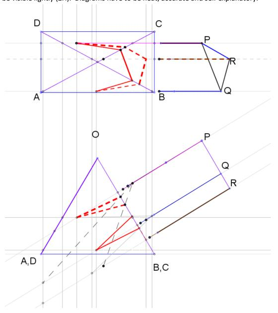
5) A building top view is shown below. Its height information is given in the side diagram. Draw the perspective view of the building.
