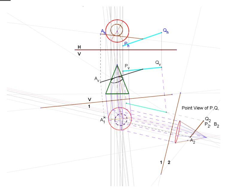
3) Triangle ABC and Vertices of D and E of Triangle DEF are given. F is constrained to be on line PQ. Find the vertex F of the triangle DEF such that it is perpendicular to triangle ABC. Clearly mark all the Edge view (EV), True Shapes (TS), true lines (TL), point views (PV)
