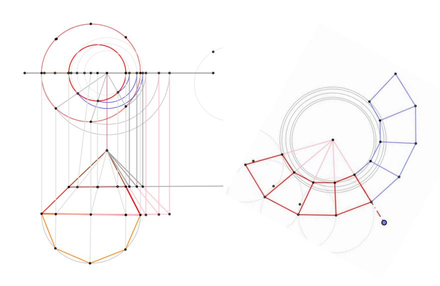
2) A line AB is drawn from given point A while B on the line PQ. The line is drawn such that it just passes by the cone and touching it. Find the point B and the line. All construction lines should also be visible lightly (2H). Diagrams have to be neat, accurate and self explanatory
